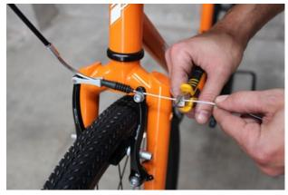
**8.** Trim the excess cable with pliers or cable cutters.
