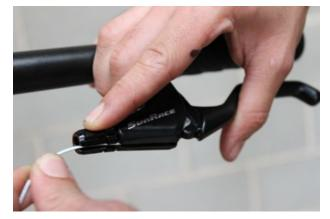
**2.** Squeeze the brake lever and thread the cable through the cable tensioner slot.
