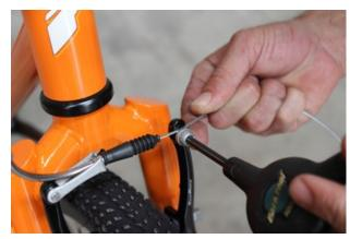
**5.** Loosen the clamp screw, thread the brake cable, and tighten it to be firm. There should be a small amount of slack, not too loose or too tight.
