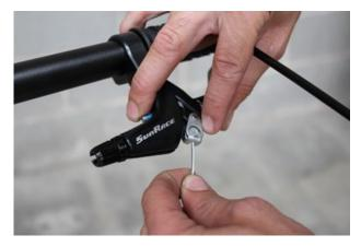
**1.** Insert the cable end into the clamp located on the brake arm.
