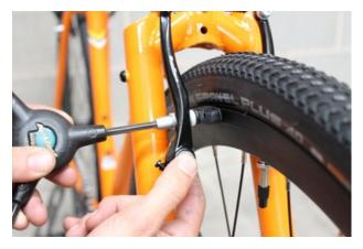
**6.** Align the brake pads with the rim's braking surface. The pads should make even contact with the rim when you squeeze the brake lever.
