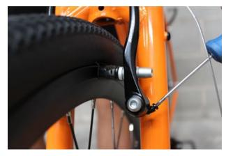
**7.** Fine-tune the cable tension using the spring adjustment screw. There is one on each side of the brake.
