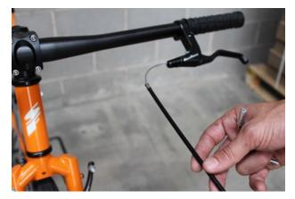
**3.** Install the cable housing.
