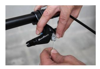
**1.** Insert the cable end into the clamp located on the brake arm.
