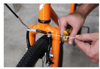
**8.** Trim the excess cable with pliers or cable cutters.
