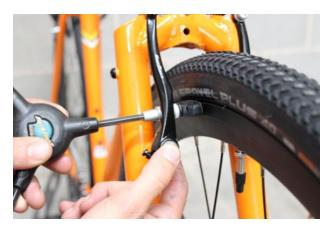
**6.** Align the brake pads with the rim's braking surface. The pads should make even contact with the rim when you squeeze the brake lever.
