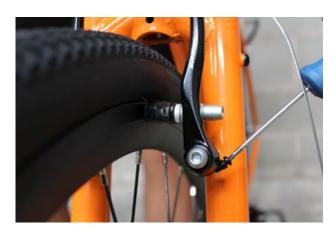
**7.** Fine-tune the cable tension using the spring adjustment screw. There is one on each side of the brake.
